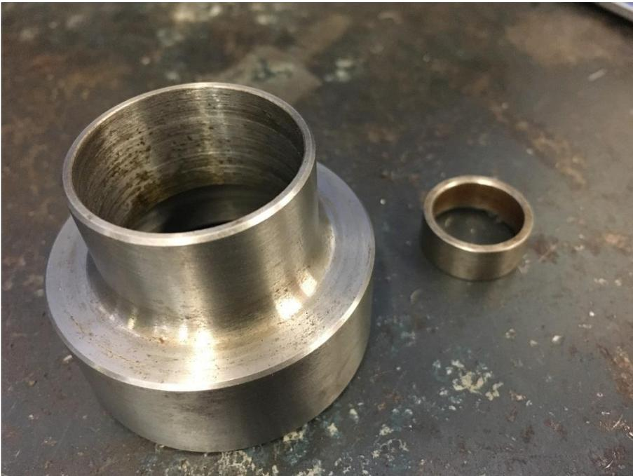
Bearing adaptor and bearing extension sleeve
