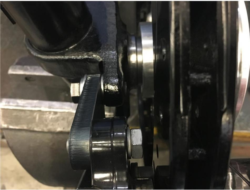
This photo shows the Caliper bolted to the Bracket and Stub axle using the spacers shown above
