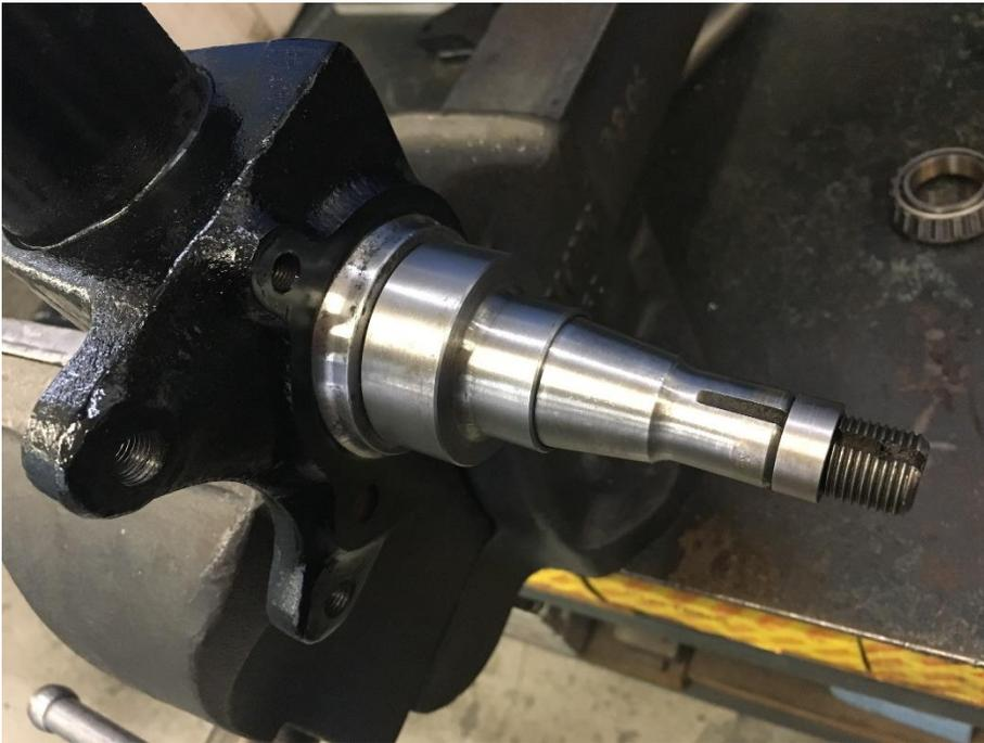
The bearing extension sleeves can now be fitted to the stub axles
