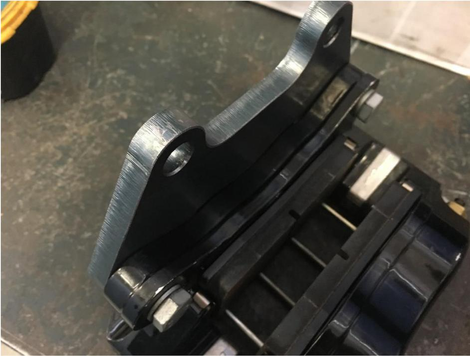
Bolt caliper to the Bracket using the supplied bolts and washers
