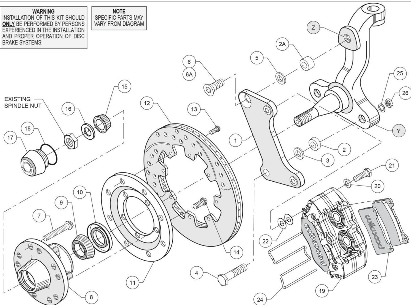
NOTE: OPTIONAL DRILLED/SLOTTED ROTOR SHOWN FOR REFERENCE PURPOSES
