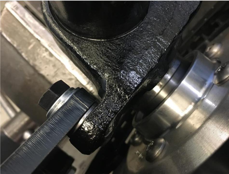
The Spacer will need to be fitted to the stub axle side then the caliper bracket and bolted using the Supplied bolts flat & spring washers
